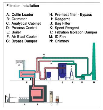
Hot gases leaving the cremator are cooled to around 120°C by passing through a Flue Gas Cooler (E) filled with a glycol/water mixture which is continuously circulated through an Air Blast Cooler (F) to dissipate excess heat to atmosphere.
